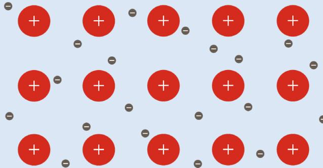
The structure of metals allows electrons to flow freely in the space between atoms. This 'sea of electrons' as seen in the image above, allows for the flow of charge through the material.
