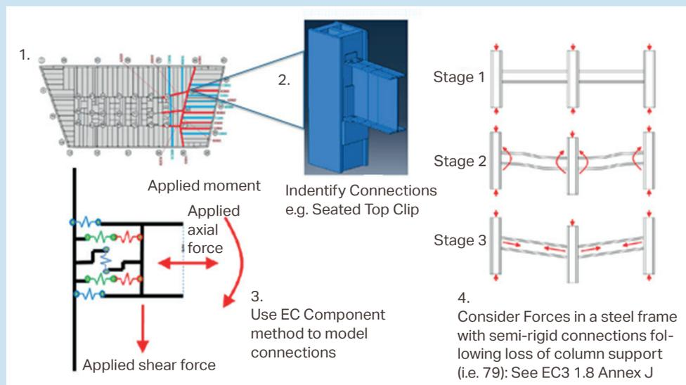
Figure 1. Wp1: East Penthouse Collapse Connections Analysis
